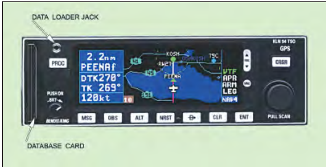
A GPS receiver used in IFR (instrument flight rules), like this Bendix-King KLN-94, must update its navigation database regularly. This can be done in two ways. A database card is inserted into the slot, or the dataloader jack connected to a PC. Updates may be obtained over the Internet.
